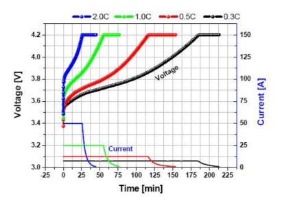
♦ Charge : CC-CV, 0.3C ~ 2.0C, 4.2V, 0.05C cut off @23 °C ±2 °C
