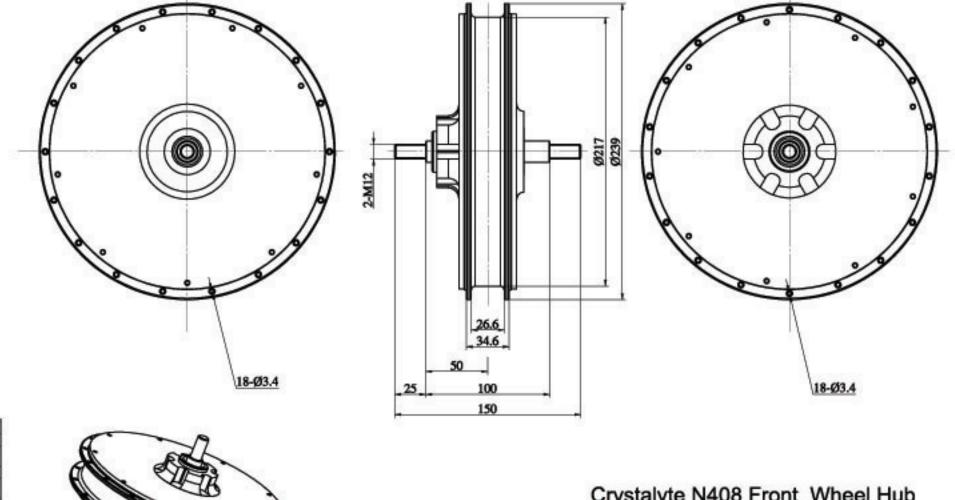
Crystalyte N408 Front Wheel Hub All dimensions are in mm unless otherwise stated
